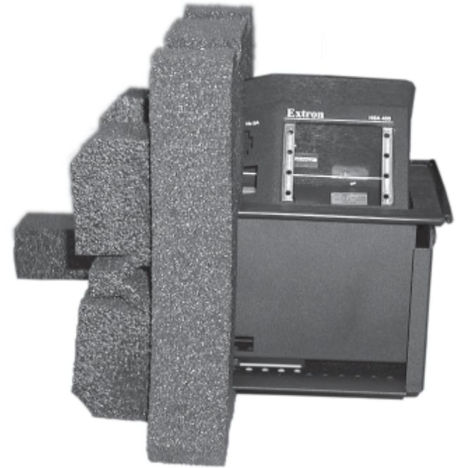
Figure B-5 — Installing the foam shell
